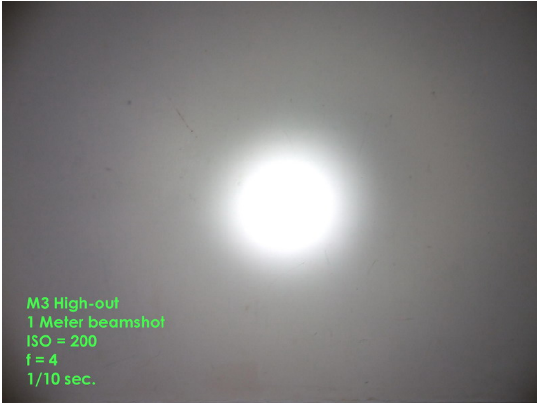
M3 drive with CR123A, Lux readings as : 900
