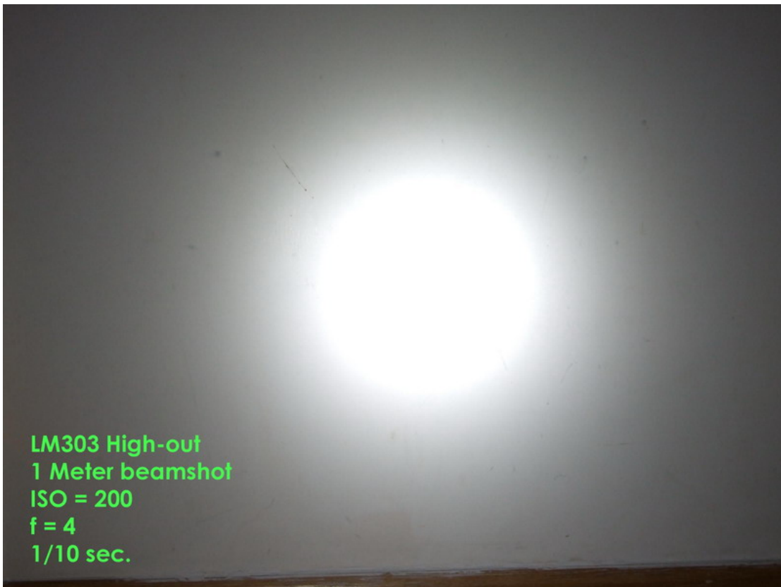
LM303 drive with rechargeable Li-ion123A Lux readings as : 1350
